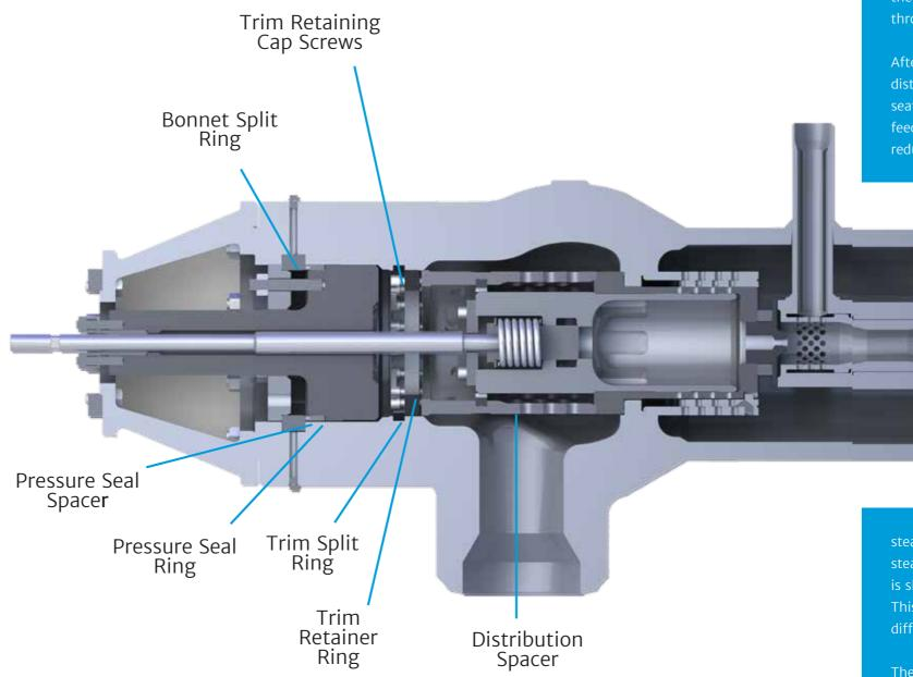
evenly positioned around the circumference. This heavy duty distribution spacer has been specifically designed to negate any upstream pipe work induced flow disturbance being communicated to the main plug. Therefore, long radius bends or isolation valves can be fitted directly to the valve inlet to minimize installation space. The main plug is fully guided by the cage and spacer to ensure complete plug stability through full travel.
