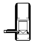
A VO-76 typically will be one nominal size smaller than the equivalent VO-II. Both will have the same size plug and internal components.
